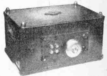
The H.T. battery eliminator of the Igranic Electric Co. A full-wave rectifier is employed and three potential outputs can be obtained.
