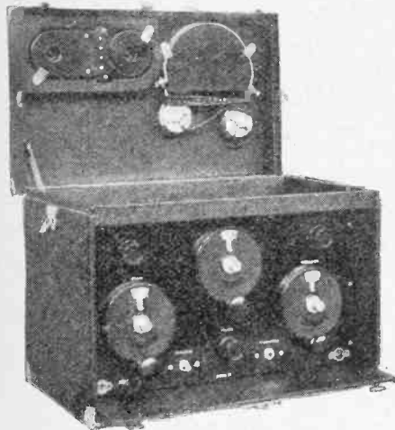
Igranic "Neutro-sonic Seven." A high-frequency amplifying stage precedes the first detector valve and a wide wavelength range is obtained by interchangeable tuning units.
