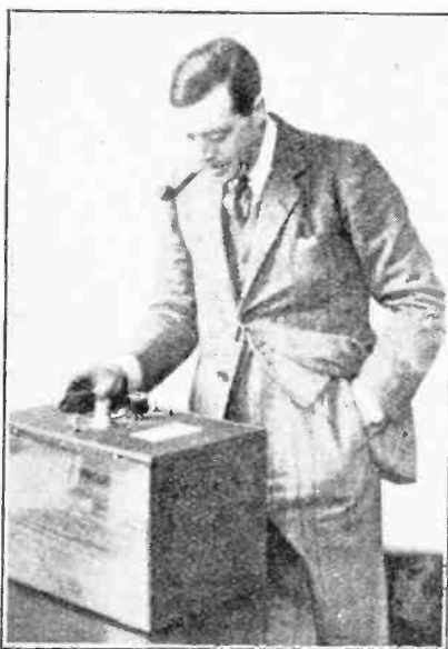
THE MAN AND THE METER. Captain P. P. Eckerstey, Chief Engineer of the B.B.C., is obviously fascinated by 2LO's new wavemeter, which has been calibrated in Brussels against a harmonic tuning fork instrument. The wavemeter was described on page 602 of our last issue.
