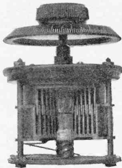
Variable condenser, fitted with concentric cylindrical plates, the moving section being operated by a quick acting thread.
